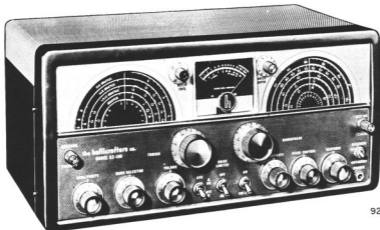
Figure 1. Hallicrafters SX-100 Receiver
