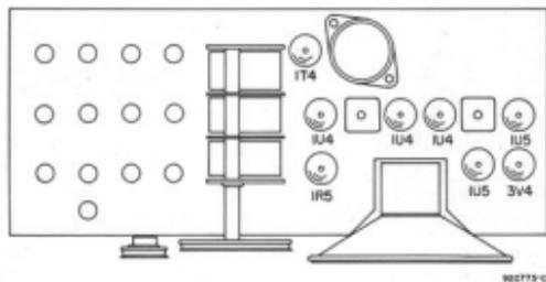
Fig. 9. Top view, location of tubes and dial lamp
